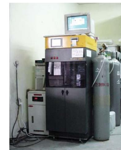
**FIGURE 7.** A BOD sensor using an MFC.
