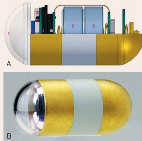
**FIGURE 1.** A: Schematic diagram of capsule endoscope: optical dome (1) lens (2), LEDs (3), image sensor (4), battery (5). B: Photograph of MiRO
