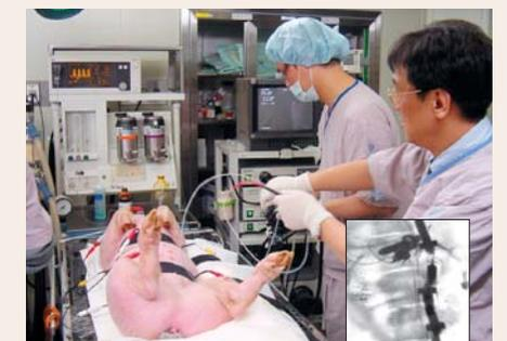
**FIGURE 5.** *In vivo* test and still image captured from X-ray movie of moving capsular micro-robot in large intestinal tract
