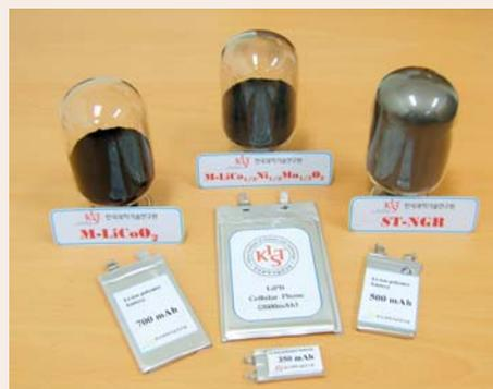
FIGURE 1. Lithium secondary batteries and electrode materials developed at KIST.
