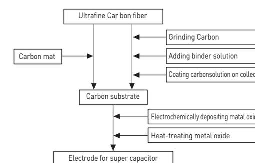
This patent discloses an improved electrode for a supercapacitor. The electrode is comprised of: (1) a collector; (2) a carbon substrate disposed on the collector consisting of ultrafine carbon fibers having a specific surface area of at least 200 m<sup>2</sup>/g (BET) and a d<sub>002</sub> value of 0.36 nm or less; and (3) a metal oxide thin layer formed on the carbon substrate.
