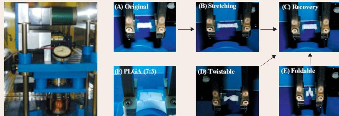
**FIGURE 1.** Bioreactor and elastic behaviors of PLCL scaffolds. PLCL scaffolds (A) were extended to 250% of their initial length (B) with 3MPa for 5 sec and recovered (C) by releasing the load. The scaffolds were twisted (D) and folded (E) via cyclic strain apparatus. PLGA (F) was broken at 20% strain.
