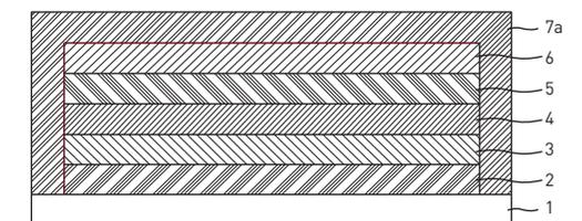
This patent discloses (1) an inorganic thin layer which is moisture and oxygen proof and composed of an inorganic composite containing at least two kinds of inorganic materials; (2) an organic electroluminescence device including the inorganic thin layer as a passivation layer; and (3) a fabrication method thereof.
