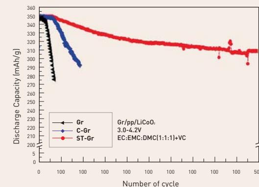
**FIGURE 4.** Cycle performance of surface-treated natural graphite anode materials compared to untreated ones.
