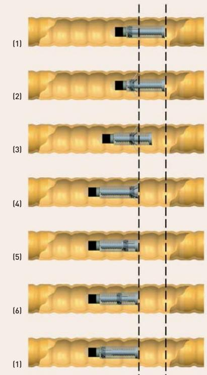
**FIGURE 3.** Locomotion principle of our proposed capsule-type micro-robot
