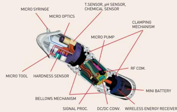
**FIGURE 6.** Conceptual diagram of future capsule endoscope to examine entire gastrointestinal tract
