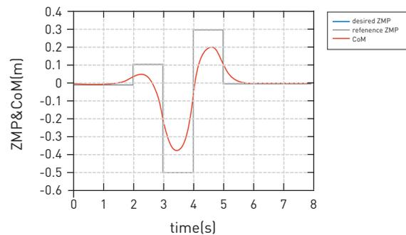
FIGURE 8. Desired ZMP trajectory
