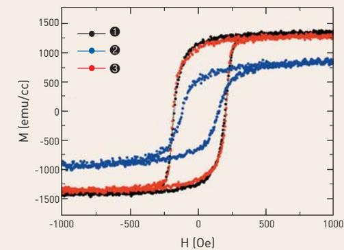
**FIGURE 5.** VSM measurement of Co-Al multilayers. (1) Cu capping/Co(3nm)/Cu buffer/Si sub. (2) Cu capping/Al(3nm)/Co(3nm)/Cu buffer/Si sub. (3) Cu capping/Co(3nm)/Al(84nm)/Si sub.
