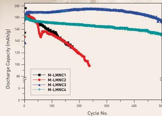
**FIGURE 3.** Cycle performance comparison of different  $\text{LiMn}_x\text{Ni}_y\text{Co}_z\text{O}_2$  cathode materials.
