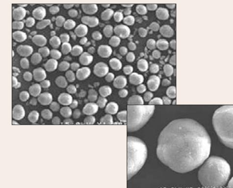
FIGURE 2. SEM image of high density cathode material with uniform morphology.
