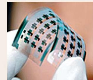
FIGURE 3. KIST's Flexible Transistor (mobility 65)
