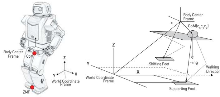
FIGURE 5. Coordinate frame FIGURE 6. Rolling sphere model for dynamic walking
