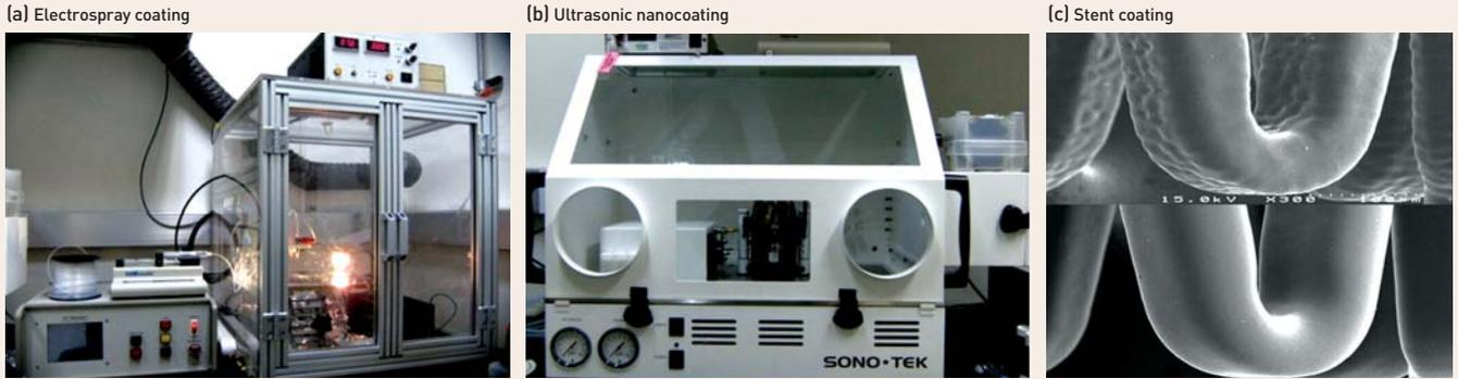
FIGURE 3. Instruments for stent coating: (a) electro spraying; and (b) ultrasonic nanocoating. The coated surface (bottom photo (c)) is extremely smooth and uniform over all surface areas as compared to one with an uneven coating (top photo (c)).
