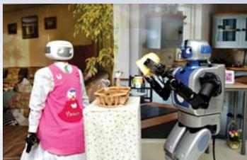
The Cognitive Robotics Center at KIST, headed by Dr. Bum-Jae You, has invented the humanoid Mahru-Z, which operates home appliances and is controlled by a remote control system in real time. Developed with highly advanced technology, Mahru-Z has the ability to walk with self-regulation and is able to find targets to operate various household machines using its own two feet and hands. Mahru-Z can also imitate a human's full body movement using a motion-capture system.
