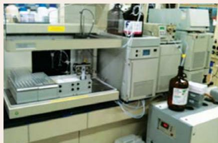
FIGURE 2. Waters FractionLynx™,MassLynx™, AutoPurification system
