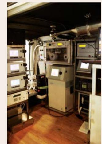
**FIGURE 5.** Multi-functional mobile laboratory for detailed monitoring of traffic-related air pollution.
