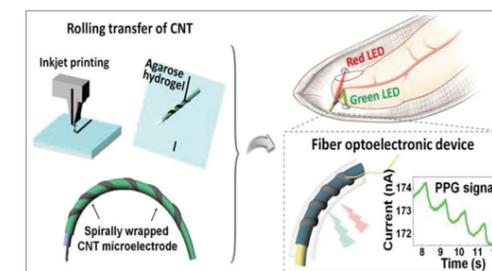
A schematic diagram of the photoelectric device implementation strategy for human signal monitoring with CNT electrode transcription
