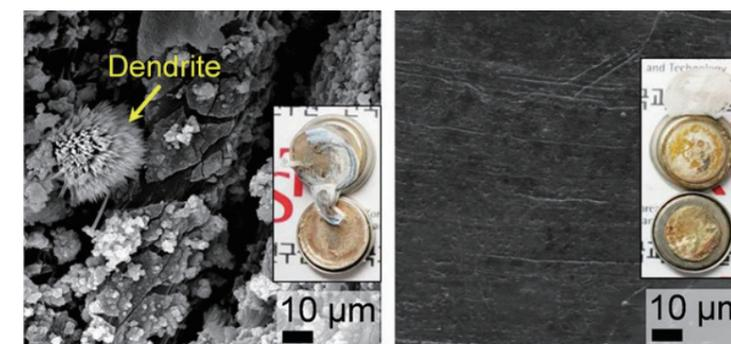
Top-view SEM images and photographs (inset) of plain-Li, and Li@p-PCL electrodes after cycling tests with Li/Li symmetrical cells at 1.0 mAcm<sup>-2</sup> and 1.0 mAhcm<sup>-2</sup>
