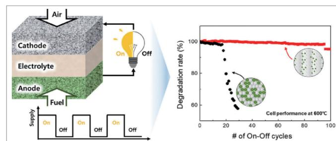
A research team in Korea has developed a ceramic fuel cell that offers both stability and high performance while reducing the required amount of catalyst by a factor of 20. The application range for ceramic fuel cells, which have so far only been used for large-scale power generation due to the difficulties associated with frequent start-ups, can be expected to expand to new fields, such as electric vehicles, robots, and drones.
