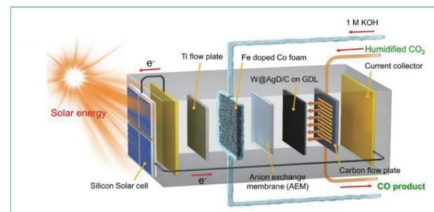
Schematic of solar-to-CO conversion system
