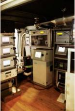
FIGURE 5. Multi-functional mobile laboratory for detailed monitoring of trafic-related air pollution.
