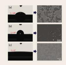
**FIGURE 1.** Photographs of water drops and SEM images of spin-coated polystyrene microspheres on (a) an as-cleaned SiO<sub>2</sub>/Si substrate, (b) a HMDScoated SiO<sub>2</sub>/Si substrate, and (c) an O<sub>2</sub>-plasmatreated SiO<sub>2</sub>/Si substrate. Contact angles are displayed in each image
