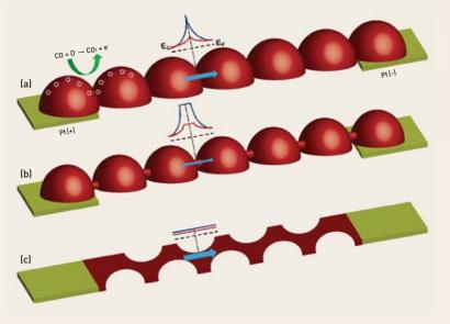
FIGURE 7. Schematic drawings of the major current path between Pt electrodes for microporous TiO<sub>2</sub> films with (a) CHH, (b) NHH, and (c) IHH.
