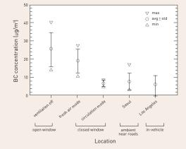
FIGURE 4. Comparison of black carbon exposure level measured in a vehicle and in ambient air. [3]
