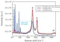
FIGURE 2. Raman spectra of the 1-10/GNSs (red), 5-10/GNSs (blue), and 5-10/GNSs after removal of the 10 by HC1 treatment (black). The graphitic peaks of GNSs disappeared when there was a thick covering of 10s (5-10/GNSs) and reappeared when the IOs on the surfaces were removed. High-Performance Micro-Solid Oxide Fuel Cells Fabricated on Nanoporous Anodic Aluminum Oxide Templates
