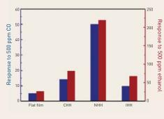
**FIGURE 6.** Responses of flat and microporous TiO<sub>2</sub> films to 500 ppm CO or ethanol.
