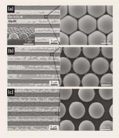
FIGURE 4. Plain-view SEM images of microporous TiO<sub>2</sub> films on Pt IDE-patterned SiO<sub>2</sub>/Si substrates (a) without O<sub>2</sub> plasma etching, or with O<sub>2</sub> plasma etching for (b) 2 min and (c) 4 min.
