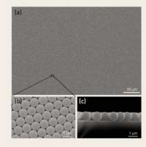
FIGURE 2. (a) Plain-view SEM image of a largearea colloid template of monolayer polystyrene microspheres on a SiO<sub>2</sub>/Si substrate. Enlarged (b) plain-view and (c) cross-sectional SEM images.
