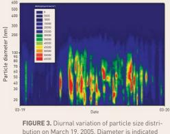
bution on March 19, 2005. Diameter is indicated on the vertical axis and particle concentration (dN/dlogD<sub>P</sub>) is represented by color contours. [8]
