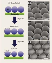
FIGURE 3. (a) A schematic drawing illustrating the link structures between polystyrene microspheres as a function of O<sub>2</sub> plasma etching time. (b-d) 52°tilted-view SEM images of microsphere templates (b) before O<sub>2</sub> plasma etching and after (c,d) O2 plasma etching for (c) 2 min and (d) 4 min.
