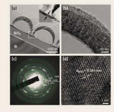
FIGURE 5. (a) Cross-sectional TEM image of isolated TiO<sub>2</sub> hollow hemispheres. (b) High magnification TEM image. (c) Selected area electron diffraction pattern. (d) High resolution TEM image.
