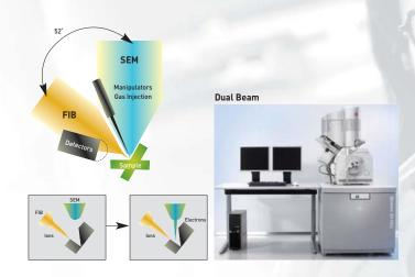
FIGURE 10. Dual-beam cryo/FIB: schematic representation and photo of the equipment used at KIST
