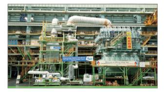
**Figure 2.** The world 1<sup>st</sup> official shop test of the LP SCR catalyst system was carried out with a marine engine of Doosan Engine co.
