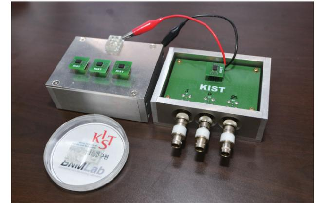
↑ The highly sensitive AI virus detection diagnostic platform, allows for immediate analysis of samples taken from the field.
