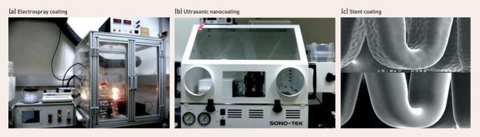
FIGURE 3. Instruments for stent coating: (a) electrospraying; and (b) ultrasonic nanocoating. The coated surface (bottom photo (c)) is extremely smooth and uniform over all surface areas as compared to one with an uneven coating (top photo (c)).
