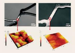
FIGURE 3. Optical images of electro-polished NiTi stent (a) before and (b) after electro-polishing.
