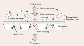
FIGURE 6. Membrane fouling phenomenon during pressure-driven separation.
