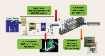
FIGURE 8. Advanced membrane process development plan for water reuse in KIST project.
