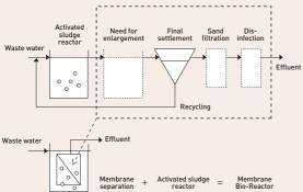
FIGURE 2. Figure 2 Application of membrane separation in a conventional wastewater treatment process in which many treatment steps (e.g., final settlement, sand filtration, and disinfection) can be replaced by a one-membrane filtration process.
