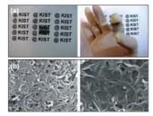
FIGURE 2. (a) Photo-images of Au NP-decorated MWCNT-HB films (Au-MWCNT-HB-2) and (b) SEM images of MWCNT (left) and Au-MWCNT-HB films (right)
