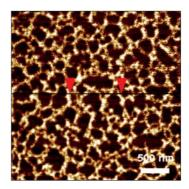
FIGURE 1. AFM image of Ultrathin film coatings of PFPE (~ 8 nm in thickness) using I-CO<sup>2</sup> as a coating solvent
