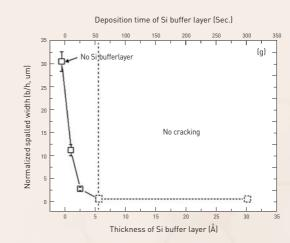
FIGURE 5. SEM images showing failure behavior as a function of the a-Si buffer layer: (a) Si buffer layer for 15 s; (b) Magnified image of square box in (a); (c) a-Si buffer layer for 30 s; (d) Magnified image of square box in (c); (e) a-Si buffer layer for 1 min; (f) Magnified image of square box in (e); (g) Spalled area width of the DLC films as a function of the a-Si buffer layer thickness: 'b' and 'h' indicate the half-width of spalled region and thickness of DLC film, respectively.
