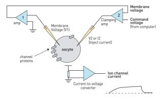
FIGURE 3. TEVC recording system and simplified electrical scheme of a TEVC setup
