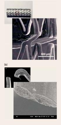
FIGURE 2. (a) Laser-cut NiTi stent; (b) Fatigue fracture on surface of nitinol stent after cyclic loading.
