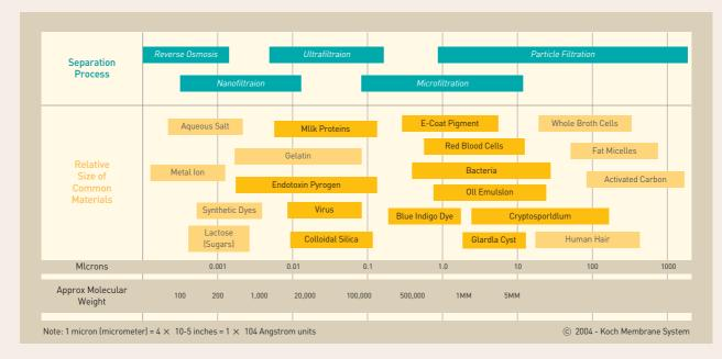
FIGURE 1. Microfiltration, ultrafiltration, nanofiltration, and reverse osmosis membrane process differing principally in the average pore diameter of the membrane filter and the different sizes of various solutes removed by each class of membrane separation (http://www.kochmembrane.com/ps\_exmem.html).
