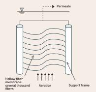
FIGURE 5. Schematics of flat-plate and hollow fiber membrane modules
