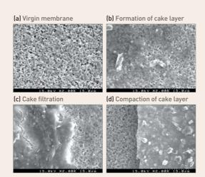
FIGURE 7. Scanning electron microscope images of membrane surfaces fouled by wastewater: (a) virgin membrane surface; (b) pore blocking is complete and cake layer (fouling layer) formation starts; (c) fouling cake filtration phase; and (d) fouling layer is concretely compacted.
