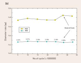
FIGURE 4. (a) Image of stent fatigue test machine; (b) Graph for long-term cyclic test.
