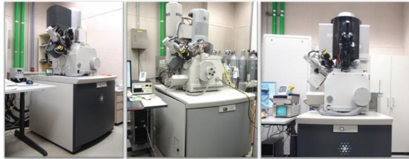
FIB equipment (FIB models: Nova600, Quanta3D, Helios)
